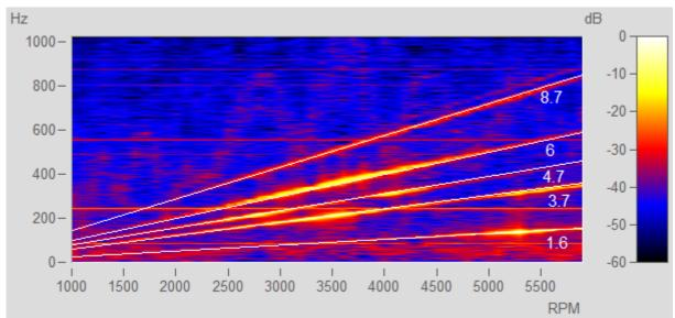
Amplitude spectrum with frequency over RPMs
