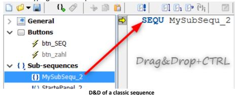
• While holding down the CTRL-key, you can use Drag&Drop on a sub-sequence to move it from the Sequences tree diagram to the input window opens the call mask of the sub-sequence functions.
