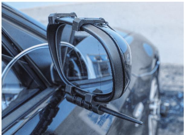
D<sup>x</sup>-antenna for mounting on side mirror
