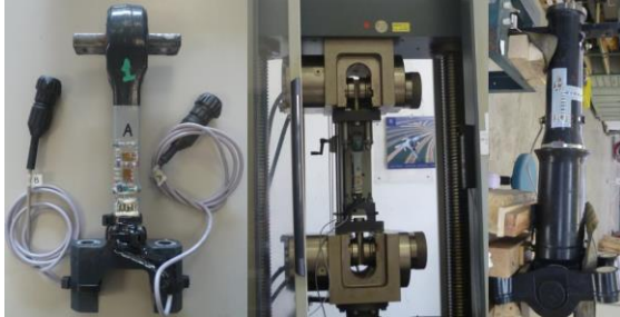
Fig. 6: Strain gauge outfitted components
